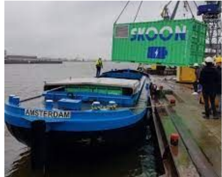
Ship exchanging into containerised battery pack to use for propulsion
